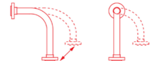
INCORRECT - Flexing movement takes place in 3 dimensions so torque is applied
