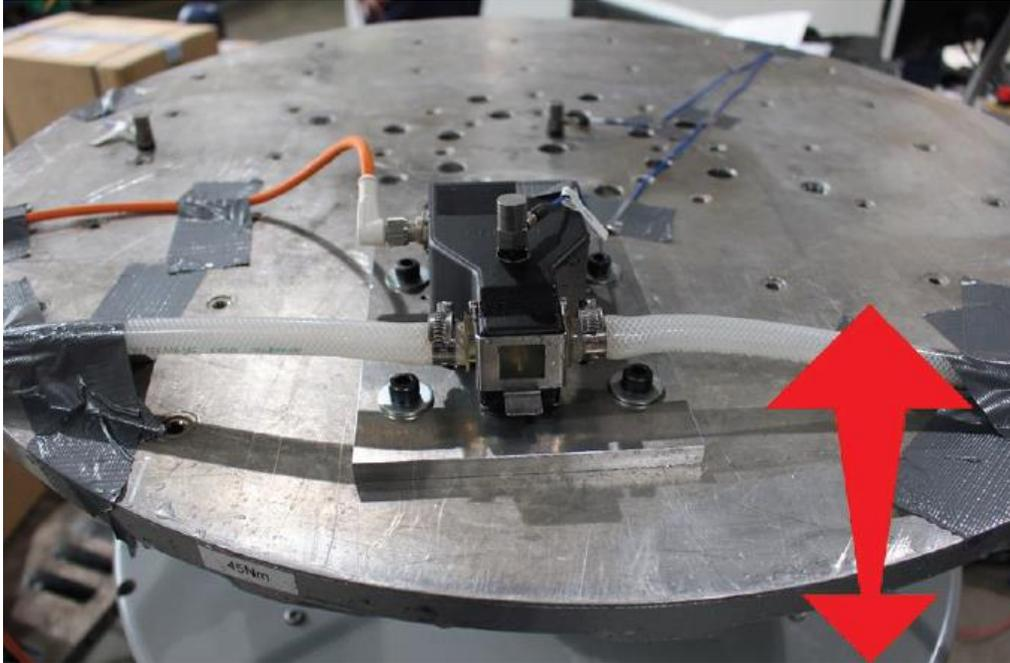
Figure 5: Photo a vibration table, here FLEXMAG mounted in Z direction.
