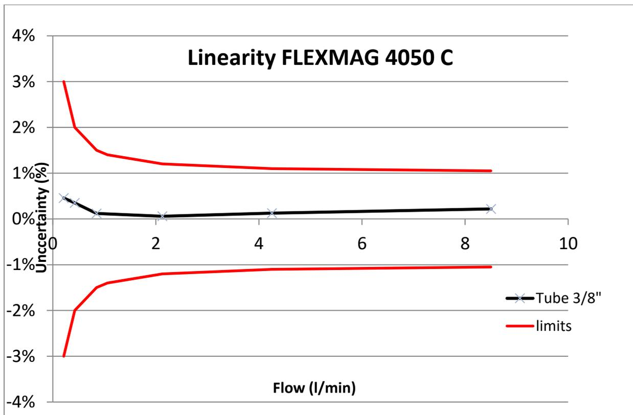
Figure 1: FLEXMAG 4050 C Accuracy
