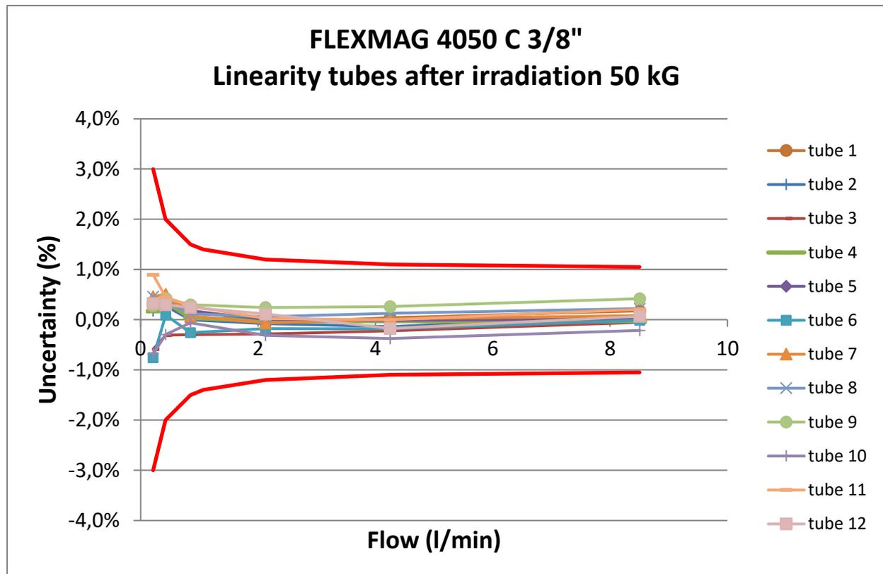
Figure 3: Accuracy after Gamma irradiation
