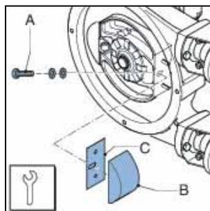
6. Fit the removed shims (C) again. Position the (new) pressing shoe (B), check that the Nord-Lock® rings (D) have been positioned correctly and tighten the retaining bolt(s) (A) a few turns. Refer to § 10.1.7.
