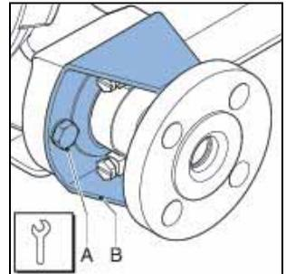
9. Position hose clamp (A) against O-ring chamber of the flange bracket (B) and fasten the retaining bolt. Make sure the bolts are tightened with the correct torque. Refer to § 10.1.7.
