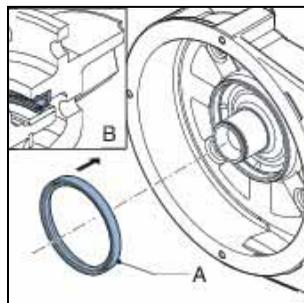
11. Check that the hub is clean and free of grease. Fit the bearings and the rings now. The bearings are placed on the hub with a slight interference fit. Use a pressing tool to press the bearings on the hub.
