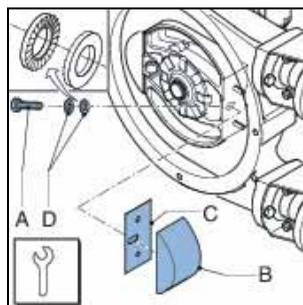
7. Check the gasket (C) for damage and replace if necessary. Refit the cover (B). Make sure that the 4 bolts (A) are refitted and that they are tightened in the correct order, diagonally opposite each other. Refer to § 10.1.7.
