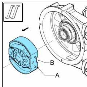
7. Dismount the retaining circlip (A) with the correct tool.
