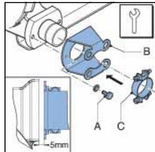
6. Slide insert (B) in flange (A) and press the insert in the hose. If necessary lubricate the insert with Bredel Genuine Hose Lubricant in order to simplify mounting. Make sure that the holes in flange (A) are aligned with the holes in flange bracket (C). Check that the insert is in the correct place. If the insert is not positioned correctly the product to be pumped may leak or the lubricant may leak.
