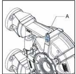
The complete hose pump, i.e. pump head, gearbox and electric motor, must be lifted using the lifting strip of the pump head plus additional support using suitably rated straps or slings (A). For the weights, refer to § 10.1.6.
