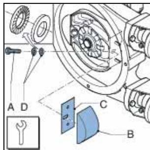
15. Check the gasket (C) for damage and replace if necessary. Refit the cover (B). Make sure that the 4 bolts (A) are refitted and that they are tightened in the correct order, diagonally opposite each other. Refer to § 10.1.7.
