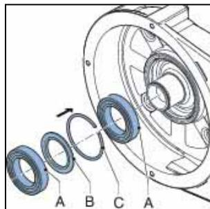
12. Mount the retaining circlip (A).
