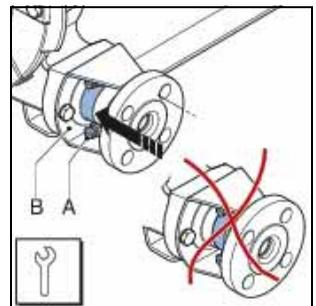
11. Fill the pump housing with Bredel Genuine Hose Lubricant. Refer to § 7.5.
