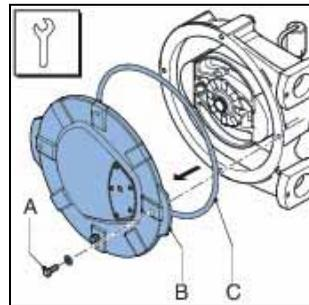
5. Loosen the retaining bolt (A) of the pressing shoe (B). Fit the shims (C) or remove them, until the correct number of shims is present. Refer to § 10.1.8.
