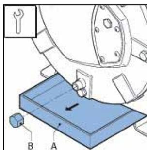
4. Remove the cover (A) by loosening the four retaining bolts (B).
