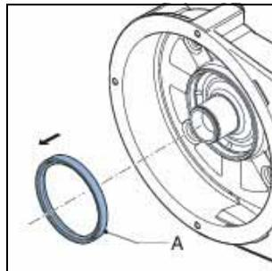
10. Fit a new seal (A) using good engineering practises. The seal must be fitted in the correct orientation (B). Make sure that the open side points to the pump cover.
