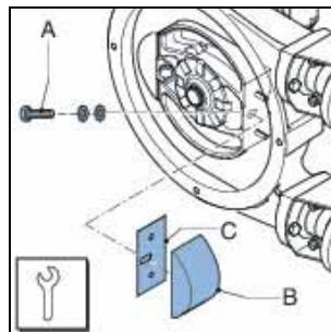
6. Refit the cover (B). Check the gasket (C) for damage and replace if necessary. Make sure that all bolts (A) are refitted and that they are tightened in the correct order, diagonally opposite each other. Refer to § 10.1.7.
