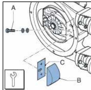
6. Extract the rotor (A) from the hub. Position both crow bars behind the recesses (B) in the rotor.
