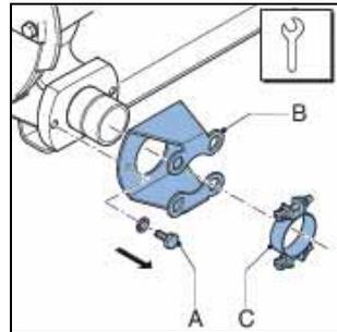
8. Slide off the sealing ring (A). Check that the sealing ring is not deformed or damaged and replace it if necessary. Carry out this procedure both for the inlet and outlet ports.
