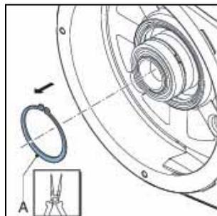
8. Dismount the bearings (A) with the correct tool, the spacer ring (B) and the retaining circlip (C).
