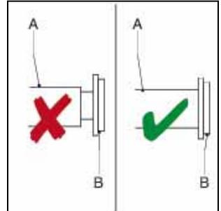
8. Now fully tighten the retaining bolts (A) of the flange bracket (B). Make sure the bolts are tightened with the correct torque. Refer to § 10.1.7.
