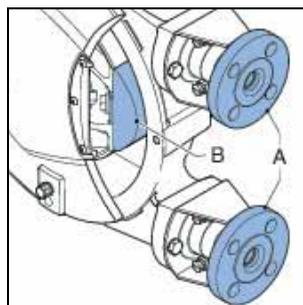
3. Place a tray (A) under the drain plug in the cover of the pump. Remove the drain plug (B). Catch the lubricant from the pump housing in the tray. Position the drain plug and tighten it firmly.
