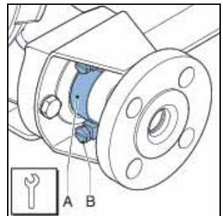
6. Pull the insert (B) from the hose and remove the flanges (A). Carry out this procedure both for the inlet and outlet ports.
