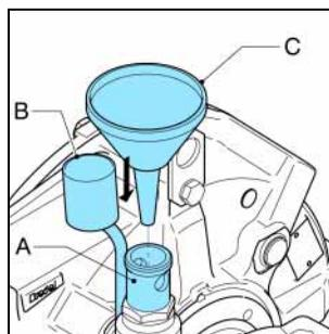
4. Keep on pouring until the lubricant level has risen at least until just above the bottom level line in the inspection window. Position the breather plug (A) and tighten it firmly.
