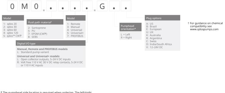
\* The pumphead side location is required when ordering. The left/right perspective assumes the user is looking at the front of the pump. The pump
